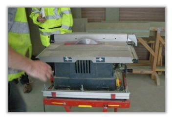
During a routine construction site inspection, this circular saw bench was seen on the site. A top guard and riving knife are required to be fitted to this type of machine. As this equipment was not available, a Prohibition Notice was served preventing use of the machine until the top guard and riving knife were fitted.
